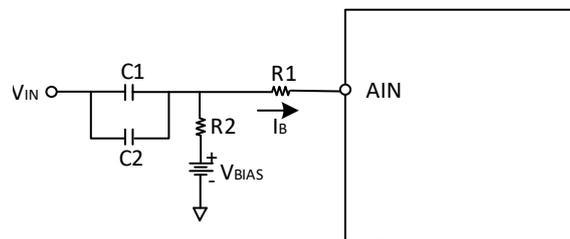
Figure 13. AC-Coupled Input
