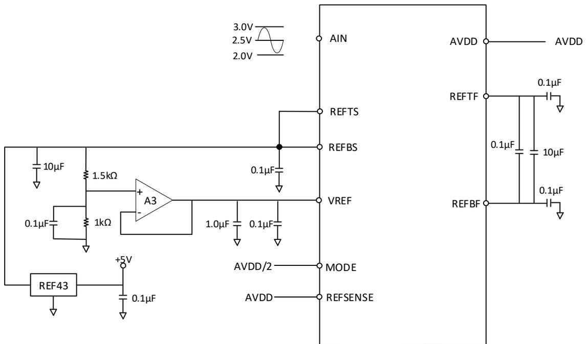
Figure 8. External Reference, 1V Input Range (Center Span Mode)
