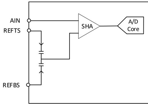
Figure 1. The MS9280 Equivalent Functional Input Circuit
