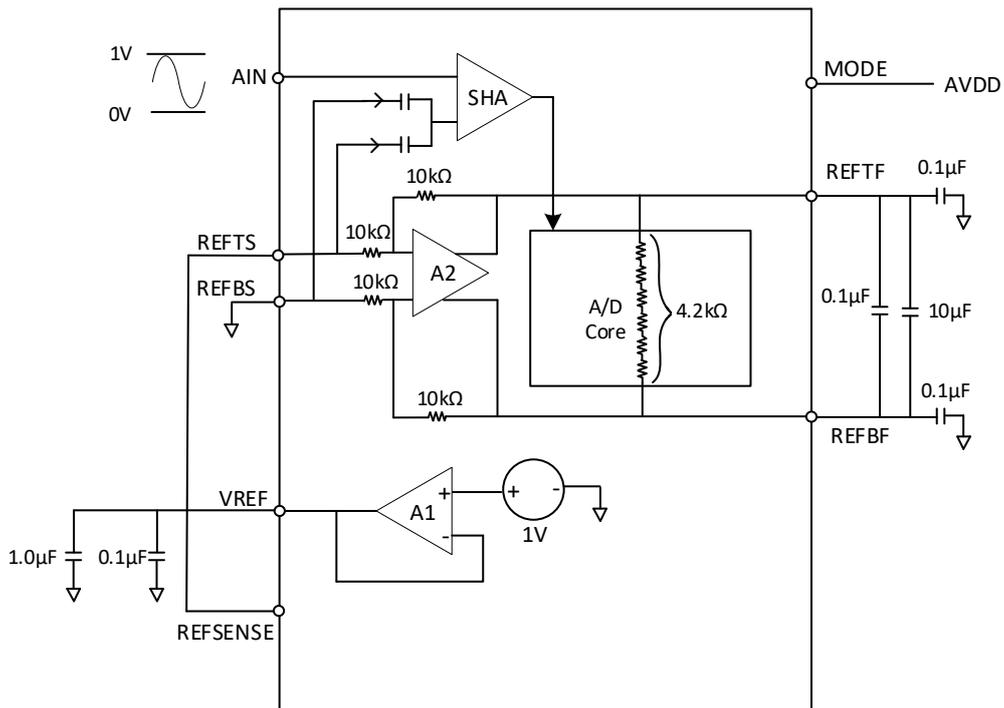
Figure 6. Internal Reference, 1V Input Range (Top/Bottom Mode)
