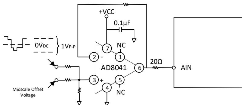
Figure 14. Bipolar Level Shift Structure
