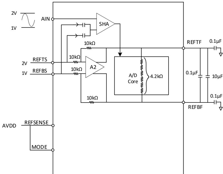
Figure 7. External Reference, 1V Input Range (Top/Bottom Mode)
