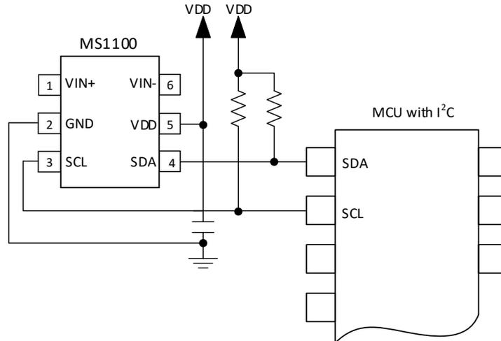
Figure 4. Typical Connections of the MS1100
