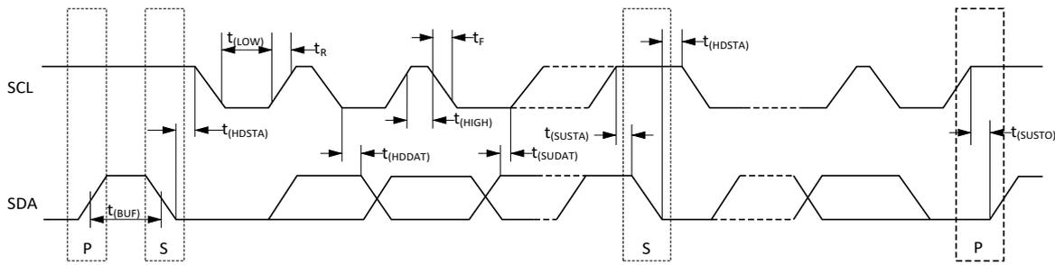
Figure 1. I<sup>2</sup>C Timing Diagram
