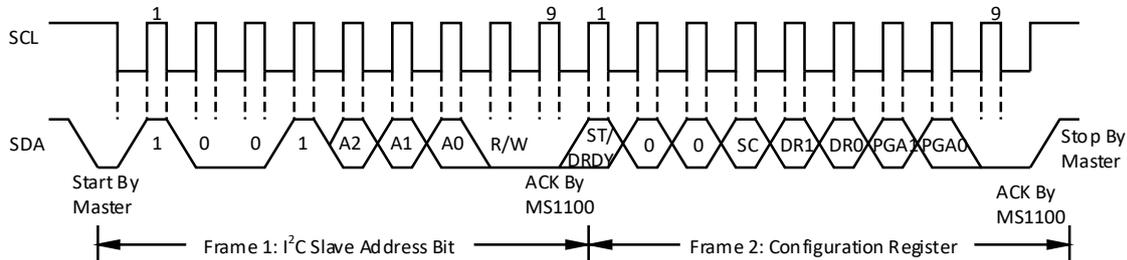
Figure 3. Timing Diagram for Writing to the MS1100
