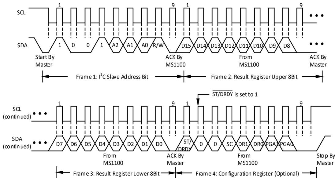
Figure 2. Timing Diagram for Reading from the MS1100
