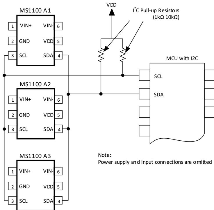
Figure 5. Connecting Multiple MS1100s
