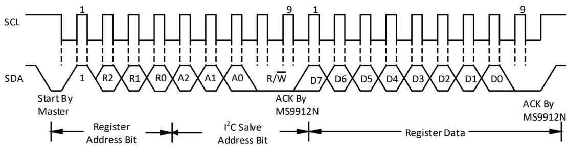
Figure 3. Timing Diagram of the MS9912N Write Operation
