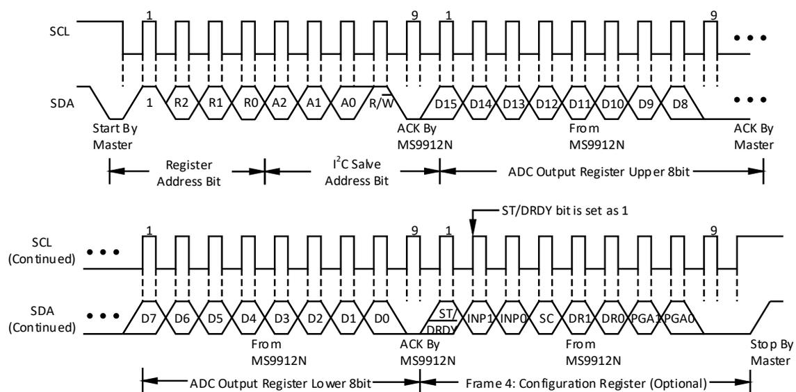
Figure 2. Timing Diagram of the MS9912N Read Operation
