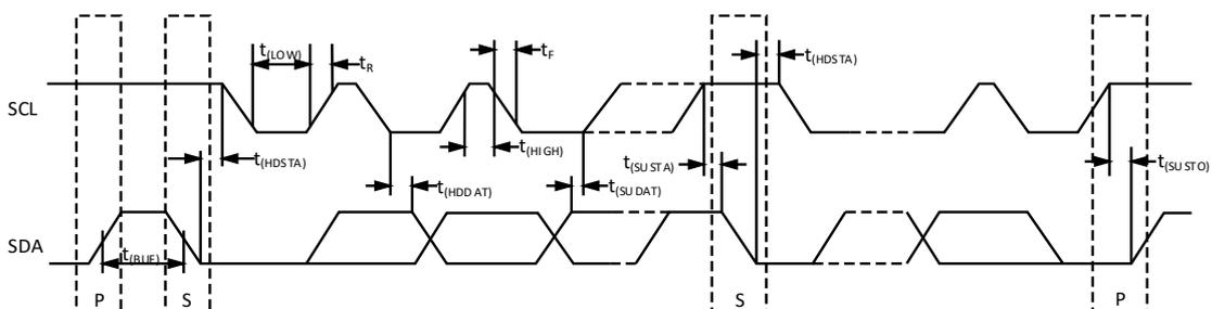
Figure 1. I<sup>2</sup>C Timing Diagram
