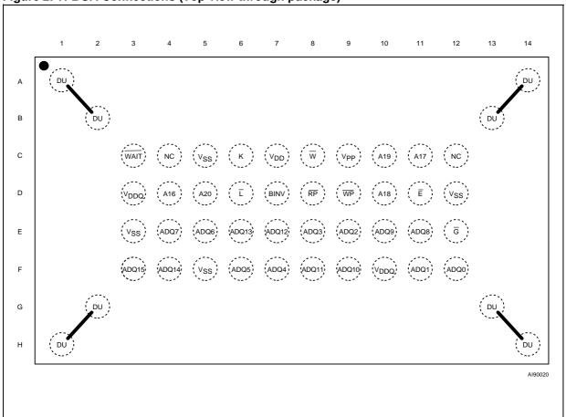
Figure 2. TFBGA Connections (Top view through package)
