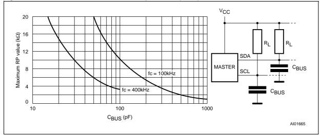
Figure 3. Maximum R<sub>L</sub> Value versus Bus Capacitance (C<sub>BUS</sub>) for an I<sup>2</sup>C Bus
