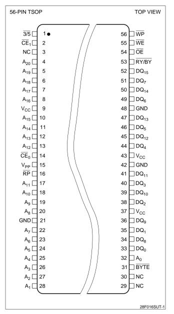
Figure 1. TSOP Configuration
