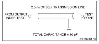
Figure 11. High Speed Transient Equivalent Testing Load Circuit (V<sub>CC</sub> = 5.0 V ± 5%)
