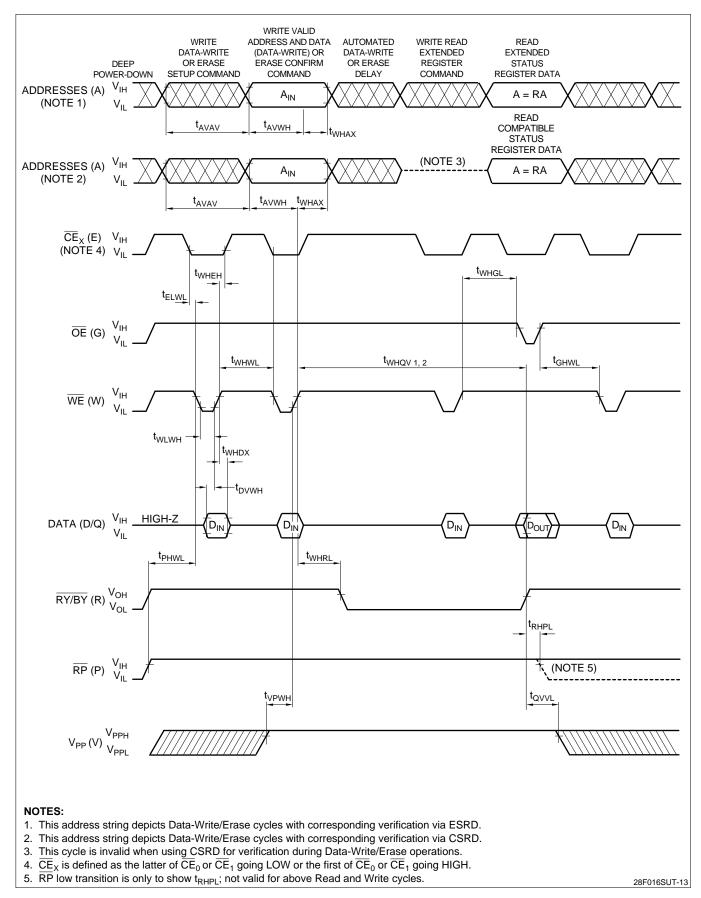
Figure 15. AC Waveforms for Command Write Operations
