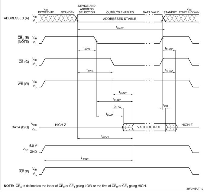
Figure 12. Read Timing Waveforms
