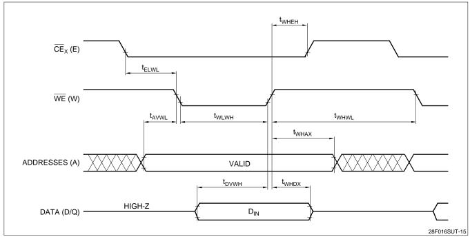
Figuer 17. Page Buffer Write Timing Waveforms
