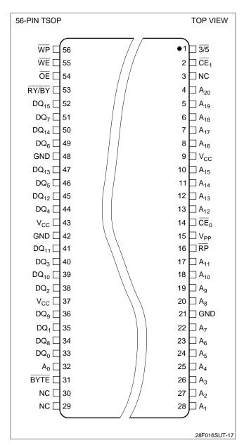
Figure 2. TSOP Reverse Bend Configuration
