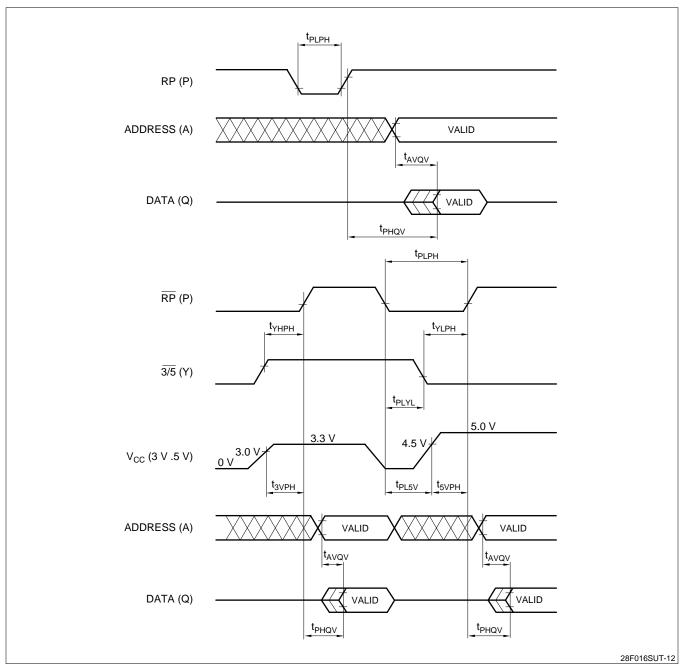
Figure 14.  $V_{CC}$  Power-Up and  $\overline{RP}$  Reset Waveforms
