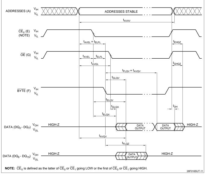
Figure 13. BYTE Timing Waveforms
