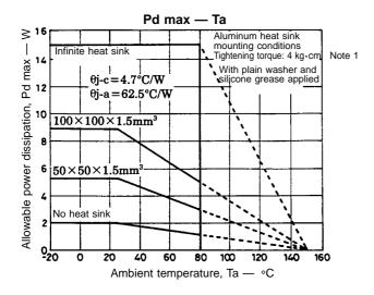
Note 1: The tightening torque referred to in the above figure is a condition specified for the heat dissipation characteristics and not a working condition to be met when mounting the heat sink.
