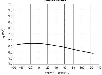
Figure 7. LT1585A Adjust Pin Current vs
