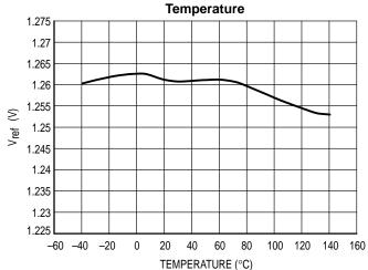
Figure 5. LT1585A-1.5 Output Voltage vs Temperature
