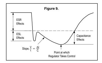
The use of capacitors with low ESR, low ESL and good high frequency characteristics is critical in meeting the output voltage tolerances of these high speed microprocessors. These requirements dictate a combination of high quality, surface mount tantalum capacitors and ceramic capacitors.
