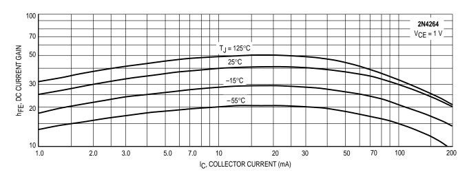
Figure 2. Minimum Current Gain
