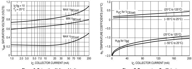
Figure 6. Saturation Voltage Limits
