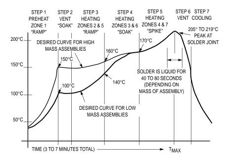
Figure 7. Typical Solder Heating Profile
