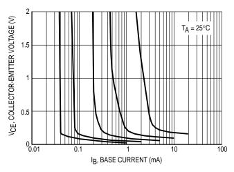
Figure 3. Collector Saturation Region
