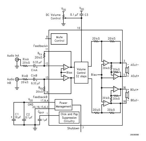
FIGURE 2. Typical Application Circuit
