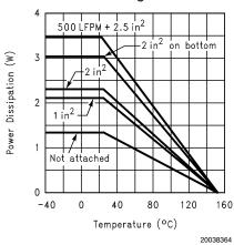
Note 17: These curves show the thermal dissipation ability of the LM4843MH at different ambient temperatures given these conditions: 500LFPM + 2in<sup>2</sup>: The part is soldered to a 2in<sup>2</sup>, 1 oz. copper plane with 500 linear feet per minute of forced-air flow across it.
