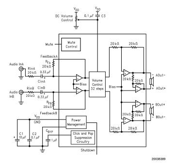
FIGURE 1. LM4843 Block Diagram
