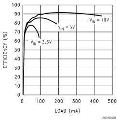
Efficiency vs Load (V<sub>OUT</sub> = 35V) - "Y"
