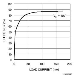
Efficiency vs Load (V<sub>OUT</sub> = 15V) - "Y"
