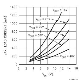
Max. Load Current vs V<sub>IN</sub> - "Y"
