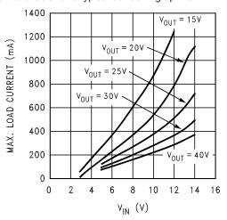
Max. Load Current vs V<sub>IN</sub> - "X"
