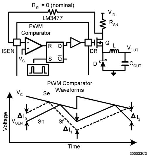
**FIGURE 4. The Current Sensing Loop and Corresponding Waveforms**
