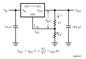
FIGURE 1. Basic Adjustable Regulator
