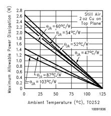
FIGURE 10. Maximum Allowable Power Dissipation vs.
