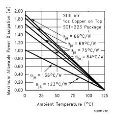
FIGURE 9. Maximum Allowable Power Dissipation vs.
