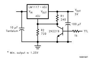
5V Logic Regulator with Electronic Shutdown\*
