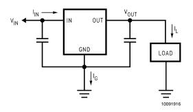
FIGURE 6. Power Dissipation Diagram
