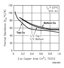
FIGURE 8.  $\theta_{\text{JA}}$  vs. 2oz Copper Area for TO-252
