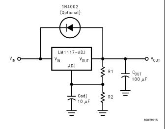
FIGURE 4. Regulator with Protection Diode
