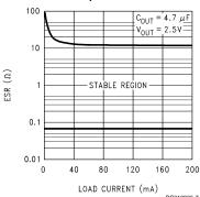
**IMPORTANT:** The output capacitor must maintain its ESR in the stable region *over the full operating temperature range of the application* to assure stability.
