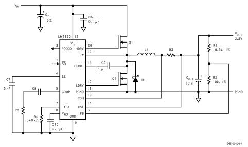
FIGURE 2. The Typical 2.5V Application Circuit
