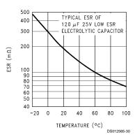
FIGURE 15. Capacitor ESR Change vs Temperature
