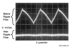
FIGURE 17. Post Ripple Filter Waveform
