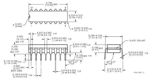
16-Lead Ceramic Dual-in-Line Package (J)
