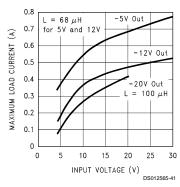
FIGURE 26. Inverting Regulator Typical Load Current
