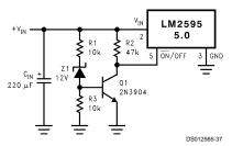
FIGURE 22. Undervoltage Lockout for Buck Regulator
