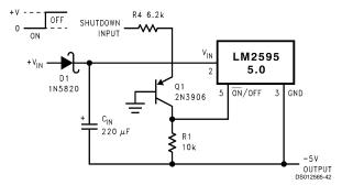
FIGURE 27. Inverting Regulator Ground Referenced Shutdown
