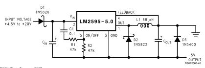
C<sub>IN</sub>: — 220 μF/25V Tant. Sprague 595D 120 μF/50V Elec. Panasonic HFQ C<sub>OUT</sub>: — 22 μF/20V Tant. Sprague 595D 120 μF/25V Elec. Panasonic HFQ
