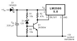
This circuit has an ON/OFF threshold of approximately 13V.
