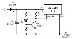
This circuit has hysteresis Regulator starts switching at  $V_{IN}$  = 13V Regulator stops switching at  $V_{IN}$  = 8V
