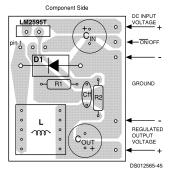
$C_{\text{IN}}$  - 150  $\mu\text{F},$  50V, Aluminium Electrolytic Nichicon, "PL series"  $C_{OUT}$  - 120  $\mu\text{F},\,25\text{V}$  Aluminium Electrolytic Nichicon, "PL series"
