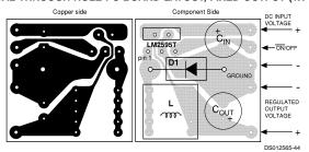
$C_{\text{IN}}$  - 150  $\mu\text{F}$ , 50V, Aluminium Electrolytic Nichicon, "PL series"  $C_{OUT}$  - 120  $\mu\text{F}$ , 25V Aluminium Electrolytic Nichicon, "PL series" D1 - 3A, 40V Schottky Rectifier, 1N5822
