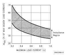
FIGURE 16. (ΔI<sub>IND</sub>) Peak-to-Peak Inductor Ripple Current (as a Percentage of the Load Current) vs Load Current
