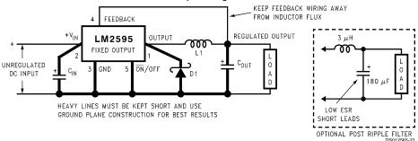
$C_{IN}$  — 120  $\mu$ F, 50V, Aluminum Electrolytic Nichicon "PL Series"  $C_{OUT}$  — 120  $\mu$ F, 25V Aluminum Electrolytic, Nichicon "PL Series" D1 — 3A. 40V Schottky Rectifier. 1N5822
