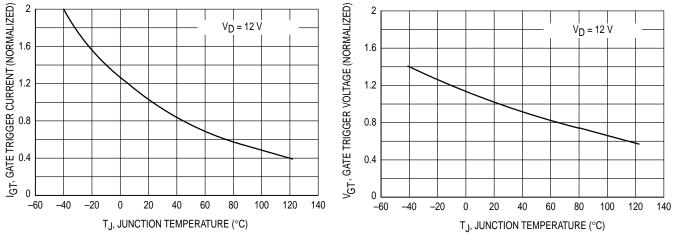
Figure 7. Gate Trigger Current versus Temperature
