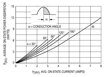
Figure 2. On-State Power Dissipation
