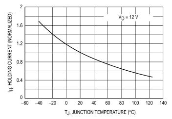
Figure 9. Holding Current versus Temperature
