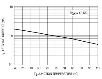
Figure 8. Typical Latching Current versus **Junction Temperature**
