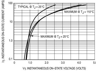
Figure 3. On-State Characteristics
