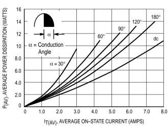
Figure 2. On-State Power Dissipation
