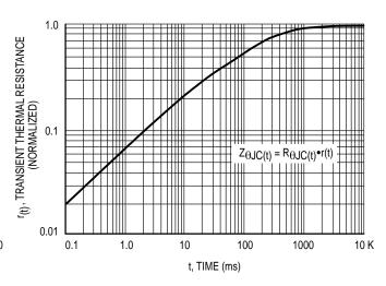
**Figure 4. Transient Thermal Response**
