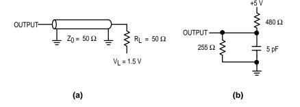
Figure 1. AC Test Loads
