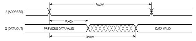
NOTE: Device is continuously selected ( $\overline{E} = V_{IL}$ ,  $\overline{G} = V_{IL}$ ).
