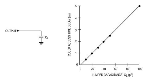
Figure 3. Lumped Capacitive Load and Typical Derating Curve
