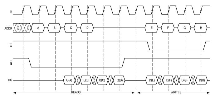
Figure 6. Configured as Non-Burst Synchronous SRAM
