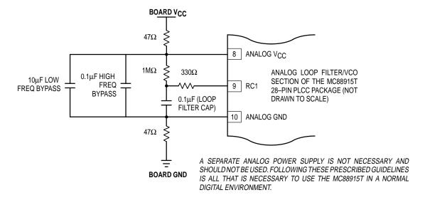
Figure 6. Recommended Loop Filter and Analog Isolation Scheme for the MC88915T
