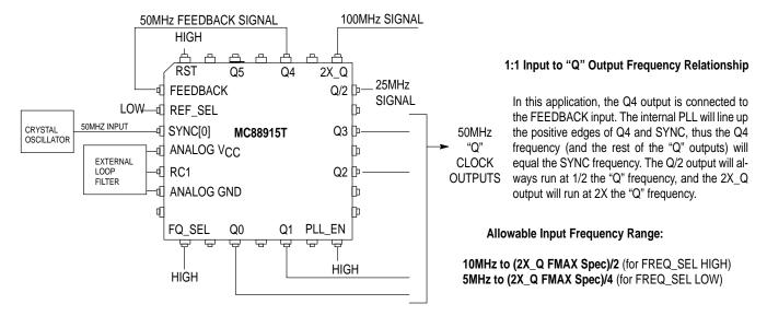
Figure 5b. Wiring Diagram and Frequency Relationships With Q4 Output Feed Back
