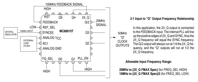
Figure 5c. Wiring Diagram and Frequency Relationships with 2X Q Output Feed Back
