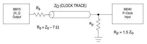
Figure 1. MC68040 P-Clock Input Termination Scheme
