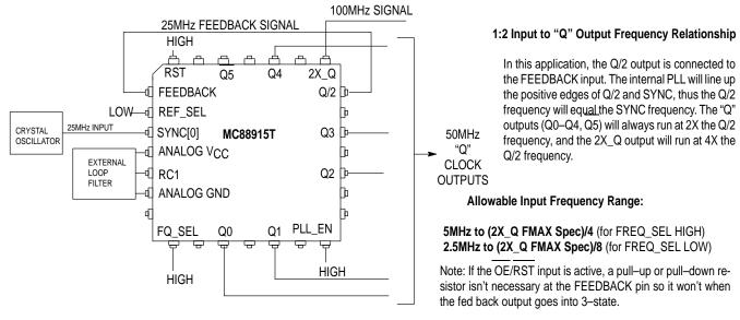
Figure 5a. Wiring Diagram and Frequency Relationships With Q/2 Output Feed Back
