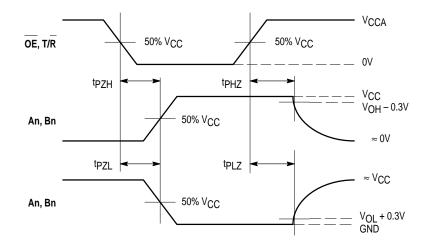
WAVEFORM 2 - OUTPUT ENABLE AND DISABLE TIMES  $t_{I\!\!R}$  =  $t_{I\!\!F}$  = 2.5ns, 10% to 90%; f = 1MHz;  $t_{W}$  = 500ns
