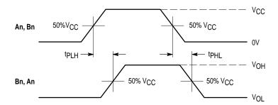
WAVEFORM 1 - PROPAGATION DELAYS  $t_R = t_F = 2.5ns$ , 10% to 90%; f = 1MHz;  $t_W = 500ns$
