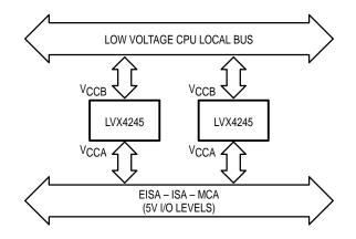
Figure 3. 3.3V/5V Interface Block Diagram
