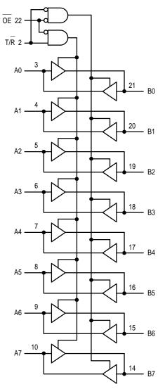
Figure 2. Logic Diagram
