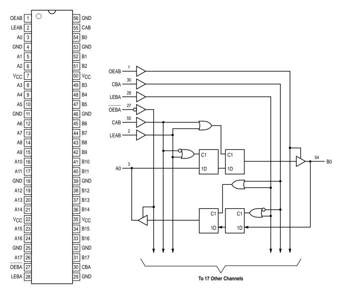
Figure 1. 56-Lead Pinout (Top View)
