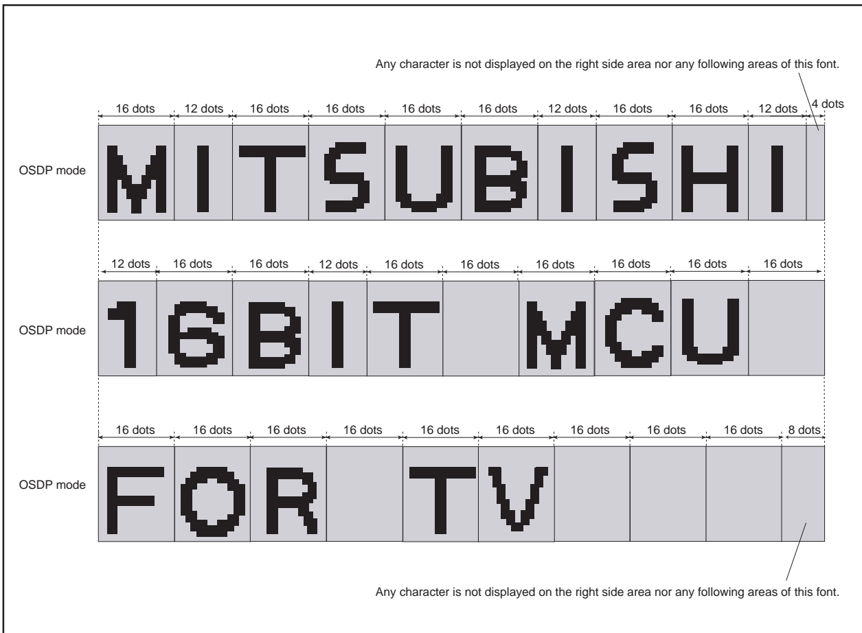
Figure 2.16.39 Display example of OSD mode block
