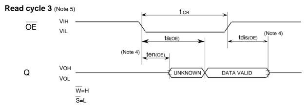
Note 5. Addresses and  $\overline{S}$  valid prior to  $\overline{OE}$  transition low by (ta(A)-ta(OE)), (ta(S)-ta(OE))
