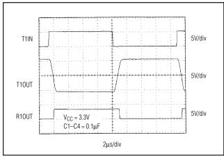
Figure 8. MAX3241E Loopback Test Result at 120kbps
