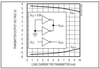
Figure 6a. MAX3241E Transmitter Output Voltage vs. Load Current per Transmitter
