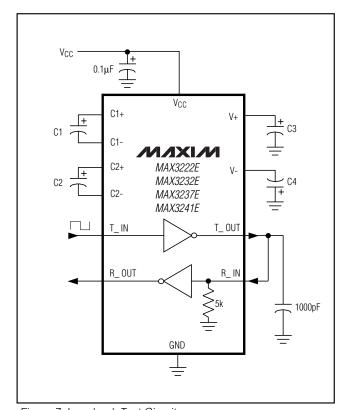
Figure 7. Loopback Test Circuit
