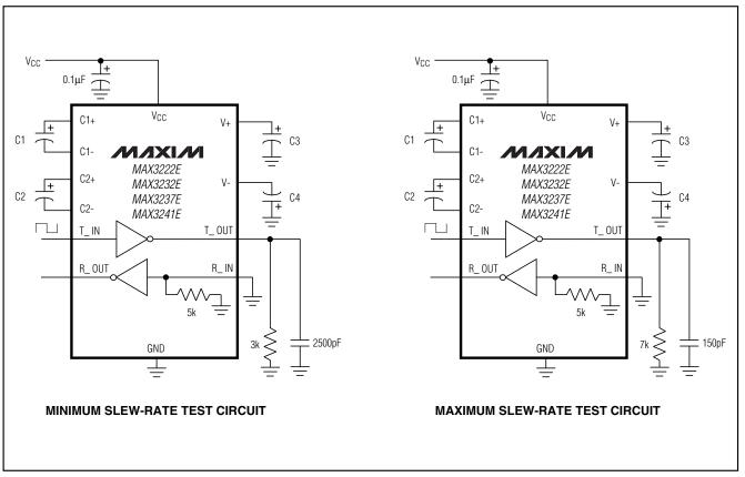
Figure 1. Slew-Rate Test Circuits
