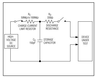
Figure 5a. IEC 1000-4-2 ESD Test Model
