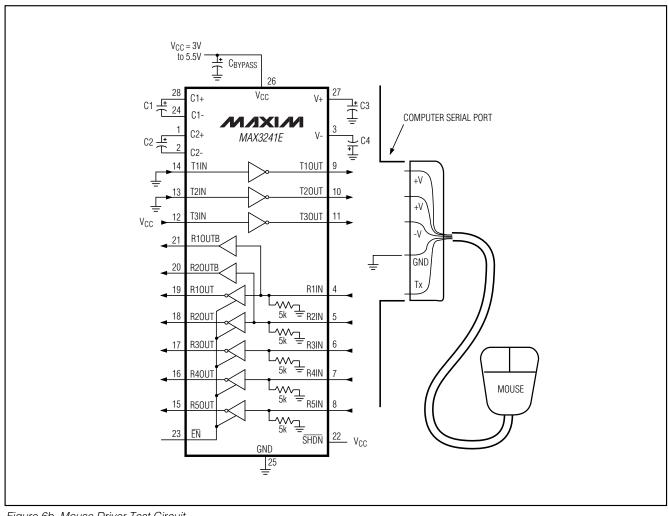
Figure 6b. Mouse Driver Test Circuit
