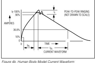
Figure 4b. Human Body Model Current Waveform
