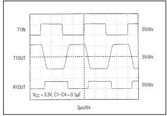
Figure 9. MAX3241E Loopback Test Result at 250kbps
