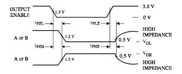
$t_{PZL}$  - S1 closed, S2 opened  $t_{PZH}$ - S1 opened, S2 closed  $t_{PLZ}$ ,  $t_{PHZ}$  - S1 and S2 closed
