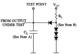
NOTES A. C<sub>L</sub> includes probe and jig capacitance. B. All diodes are 1N916 or 1N3064.
