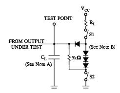
NOTES A.  $C_L$  includes probe and jig capacitance. B. All diodes are 1N916 or 1N3064.
