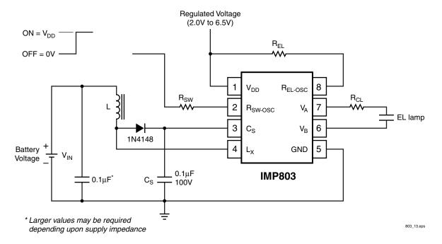
Figure 5. Dual Supply Operation
