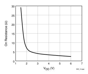
Figure 6. Boost Switch On Resistance
