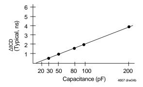
Figure 2c. Lumped Capacitive Load, Typical Derating
