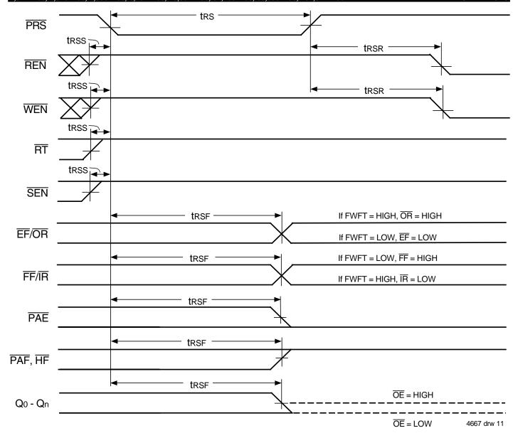
Figure 6. Partial Reset Timing
