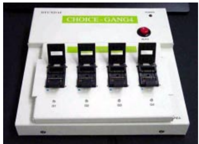
Figure 1-3 OTP Gang Programmer CHOICE-GANG4™
