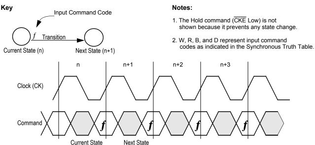
Current State and Next State Definition for Pipelined and Flow Through Read/Write Control State Diagram
