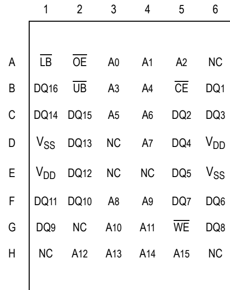
6 mm x 8 mm, 0.75 mm Bump Pitch (Package U)
