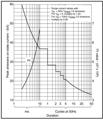
Fig.7 Surge (non-repetitive) on-state current vs time (with 50%  $V_{RSM}$  at  $T_{case}$  = 125°C)
