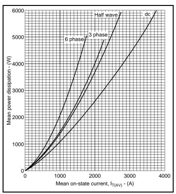
Fig.2 Maximum (limit) on-state characteristics
