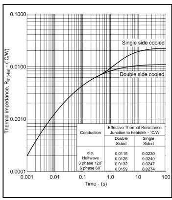
Fig.6 Transient thermal impedance - junction to heatsink
