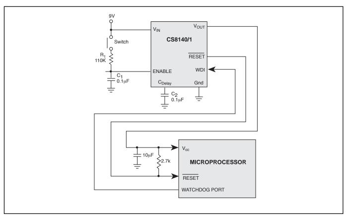
Figure 8. Applications diagram for CS8140. The CS8140 provides a 5V tightly regulated supply and control function to the microprocessor. In this application, the microprocessor controls its own power down sequence (see text).
