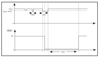
4b: Undervoltage Triggered RESET
