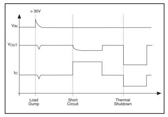
Figure 2: Typical Circuit Waveforms for Output Stage Protection.
