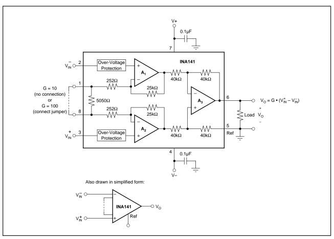
FIGURE 1. Basic Connections.
