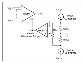
FIGURE 2. Optional Trimming of Output Offset Voltage.
