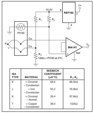
FIGURE 7. Thermocouple Amplifier With RTD Cold-Junction Compensation.
