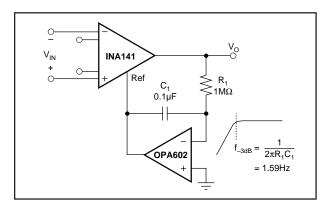
FIGURE 6. AC-Coupled Instrumentation Amplifier.
