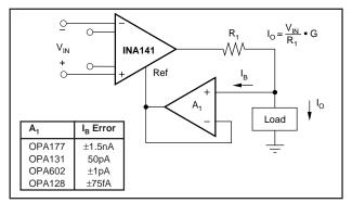
FIGURE 8. Differential Voltage to Current Converter.
