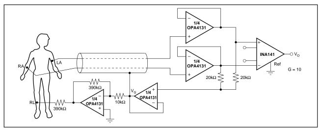
FIGURE 4. ECG Amplifier With Right-Leg Drive.
