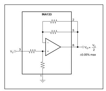
FIGURE 8. Precision Gain = 1/2 Amplifier.
