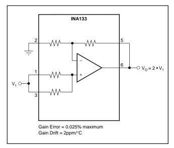
FIGURE 7. Precision Gain = 2 Amplifier.
