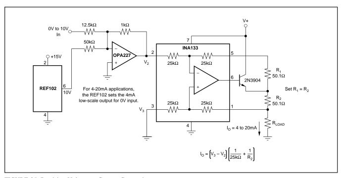
FIGURE 25. Precision Voltage-to-Current Conversion.
