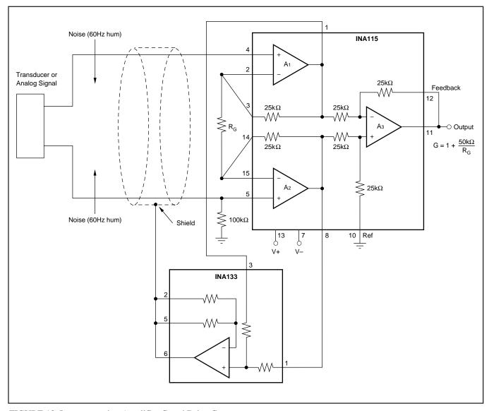
FIGURE 13. Instrumentation Amplifier Guard Drive Generator.
