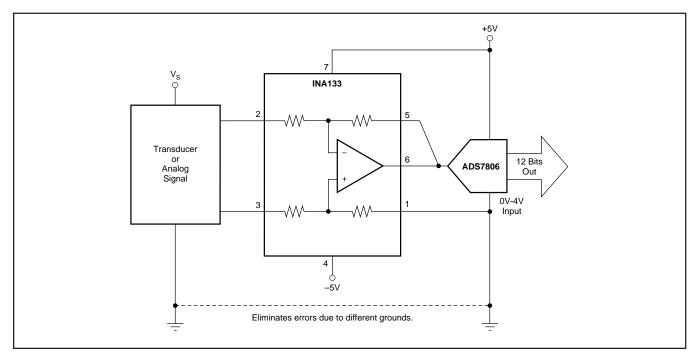
FIGURE 20. Differential Input Data Acquisition.
