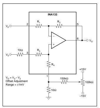
FIGURE 2. Offset Adjustment.
