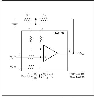
FIGURE 12. Precision Summing Amplifier with Gain.
