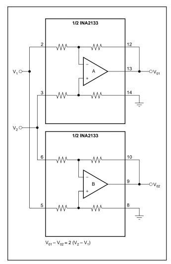
FIGURE 18. Differential Output Difference Amplifier.
