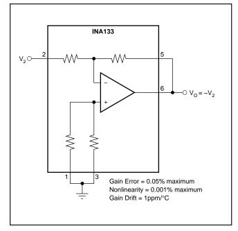
FIGURE 6. Precision Unity-Gain Inverting Amplifier.
