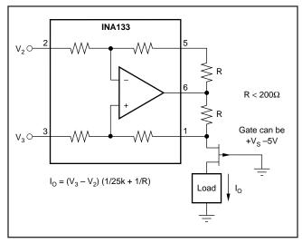
FIGURE 17. Isolating Current Source.
