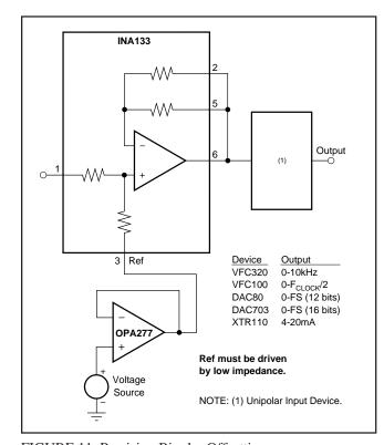
FIGURE 11. Precision Bipolar Offsetting.
