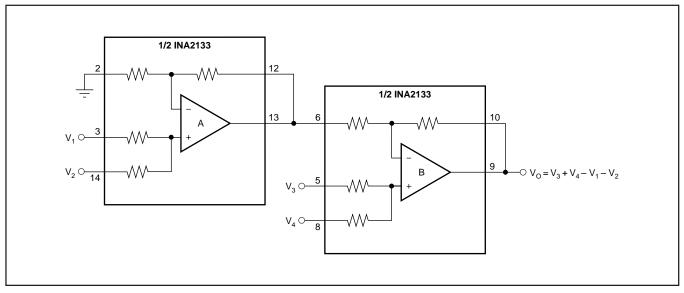
FIGURE 14. Precision Summing Instrumentation Amplifier.
