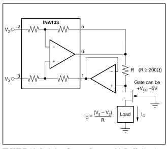
FIGURE 19. Isolating Current Source with Buffering Amplifier for Greater Accuracy.
