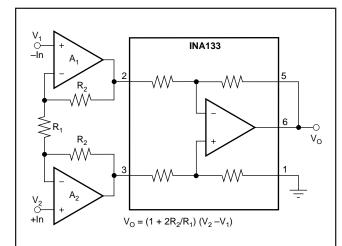
The INA133 can be combined with op amps to form a complete instrumentation amplifier with specialized performance characteristics. Burr-Brown offers many complete high performance IAs. Products with related performances are shown at the right in the table below.
