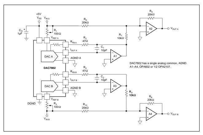
FIGURE 6. Bipolar Configuration with Gain Trim.
