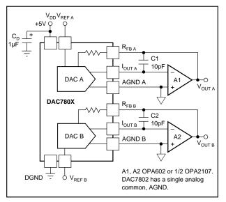
FIGURE 3. Unipolar Configuration.
