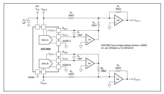
FIGURE 5. Bipolar Configuration.
