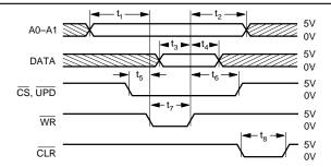
NOTES: (1) All input signal rise and fall times are measured from 10% to 90% of +5V.  $t_R = t_F = 5$ ns. (2) Timing measurement reference level is  $V_{IH} + V_{IL}$
