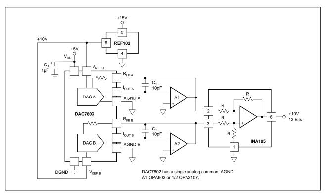
FIGURE 8. 13-Bit Bipolar DAC.
