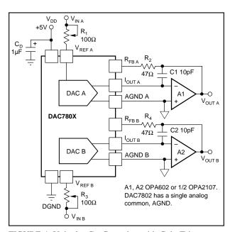
FIGURE 4. Unipolar Configuration with Gain Trim.
