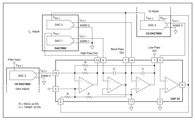
FIGURE 9. Digitally Programmable Universal Active Filter.
