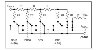
FIGURE 1. Simplified Circuit Diagram for DAC A.
