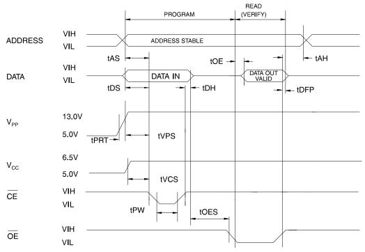
Notes: 1. The Input Timing Reference is 0.8V for  $V_{IL}$  and 2.0V for  $V_{IH}$ .
