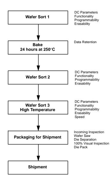
Figure 1. AMD KGD Product Test Flow
