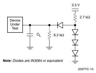
Figure 10. Test Setup
