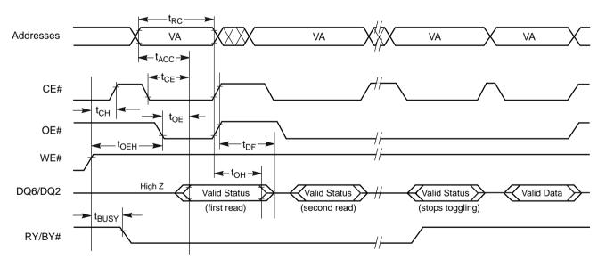
**Note:** VA = Valid address; not required for DQ6. Illustration shows first two status cycle after command sequence, last status read cycle, and array data read cycle.
