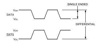
Figure 2. Data Input/Output Logic Level Definitions
