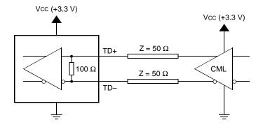
(A) TRANSMITTER INTERFACE—dc COUPLED—(CML)
